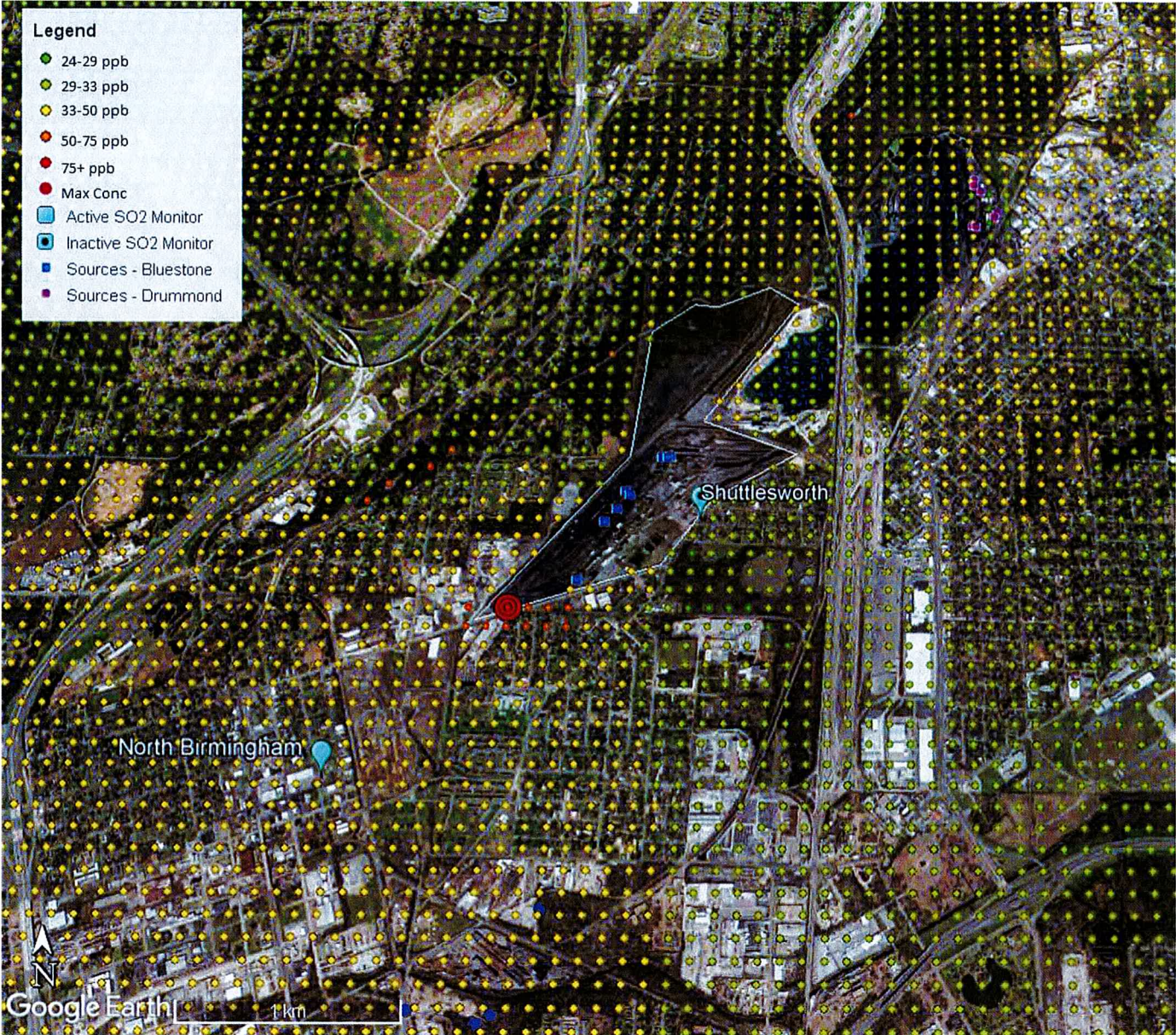
Figure 18. Run 2, Maximum Predicted 99 th Percentile Daily Maximum 1-Hour SO 2 Concentrations at Bluestone Coke's Boilers Existing Stack Heights with Emissions Reduced by 95% from 2019 Actual Emissions
