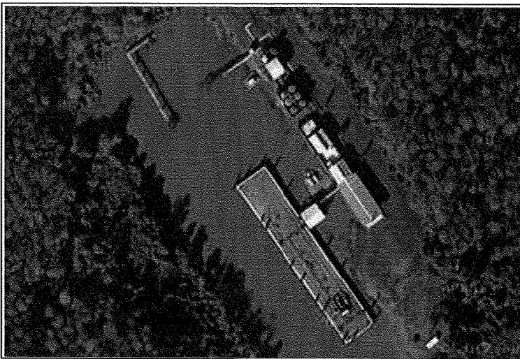
Aerial photograph of the overall well site at FAS with living quarters and a barge parked at the dock. Barges ferried wastewater from the FAS transfer station to the well site for disposal into the injection well.
